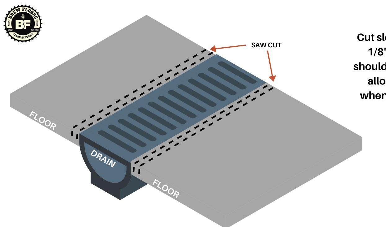
Cut slots into concrete at 1/8" W x 1/8" D. Slots should be close to drain to allow for clean finish when applying coating.
